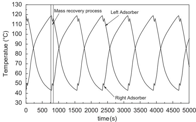
Fig. 8. Temperature profile of adsorber (720 s heating/cooling time, 60 s mass recovery time, cooling water inlet temperature: 25 °C, chilled fluid inlet temperature: −10 °C).
