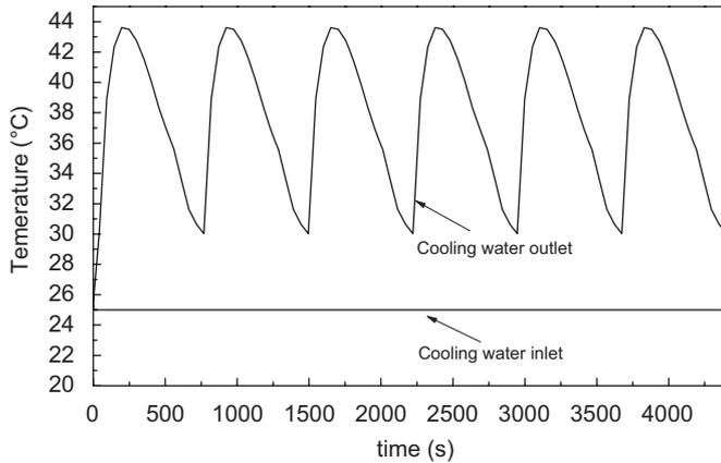
Fig. 5. Temperature profile of cooling water (720 s heating/cooling time, 60 s mass recovery time, cooling water inlet temperature: 25 °C, chilling fluid inlet temperature: -10 °C).
