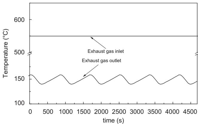
Fig. 6. Temperature profile of exhaust gas (720 s heating/cooling time, 60 s mass recovery time, cooling water inlet temperature: 25 °C, chilling fluid inlet temperature: -10 °C).
