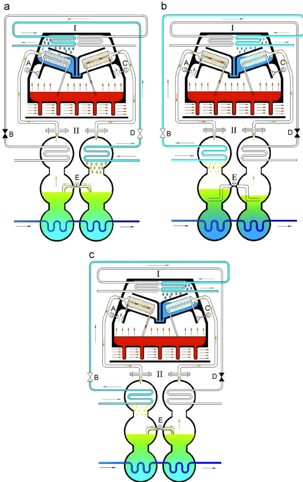
Fig. 2. (a) Mass recovery process (from right evaporator to left evaporator); (b) left adsorber in desorption phase and right adsorber in adsorption phase and (c) mass recovery process (from left evaporator to right evaporator).
