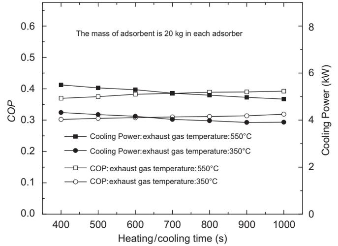
Fig. 3. Variation of the heating/cooling time with the cooling power and COP (60 s mass recovery time, cooling water inlet temperature: 25 °C, chilling fluid inlet temperature: –10 °C).
