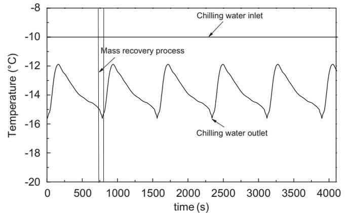
Fig. 7. Temperature profile of chilled fluid (720 s heating/cooling time, 60 s mass recovery time, cooling water inlet temperature: 25 °C, chilled fluid inlet temperature: -10 °C).
