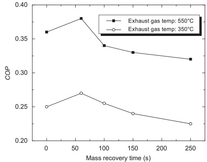
Fig. 4. Variation of the mass recovery time on the COP (720 s heating/cooling time).
