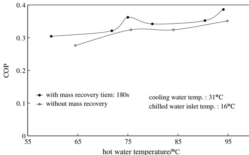
Fig. 10. Effects of the mass recovery on COP with different hot water temperature.
