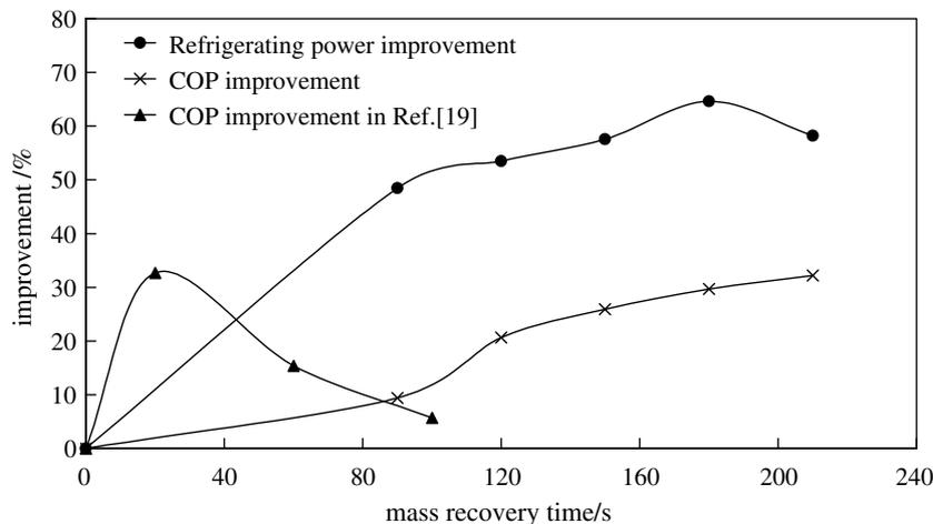
Fig. 8. Improvement of the chiller performance with different mass recovery time.
