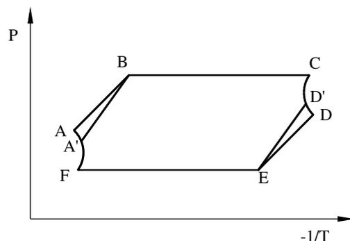
Fig. 4. Clapeyron diagram of ideal cycle.
