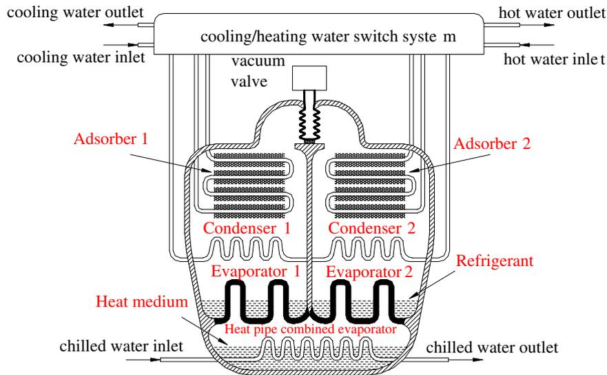
Fig. 1. Schematic diagram of the improved silica gel-water adsorption chiller.
