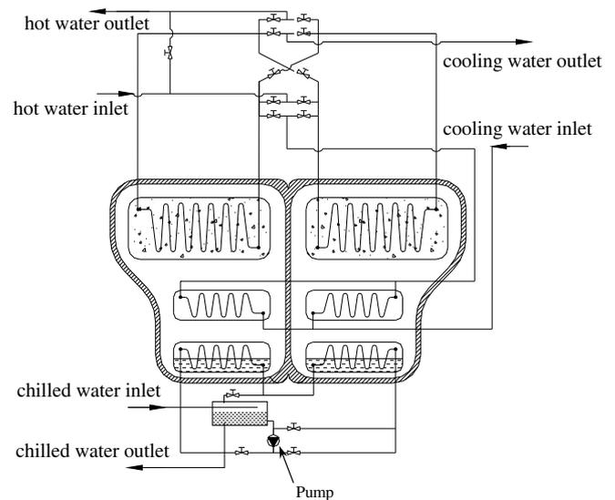
Fig. 3. The former silica gel-water adsorption chiller [19].
