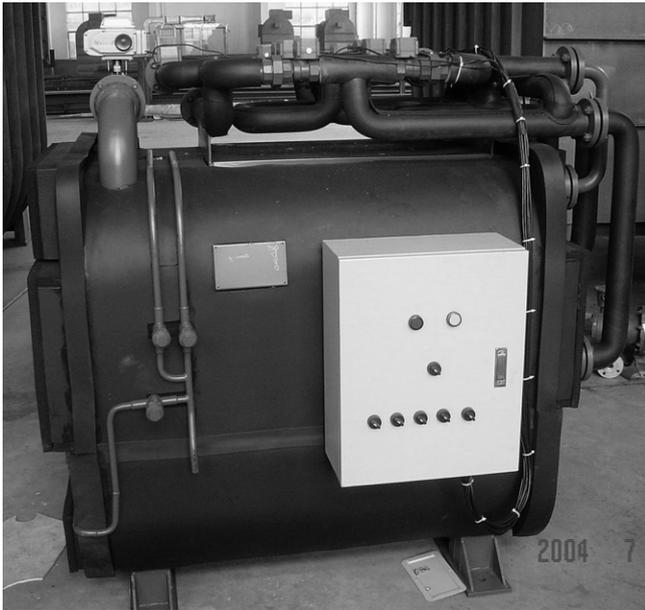
Fig. 2. Photograph of the improved silica gel-water adsorption chiller.
