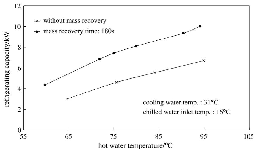
Fig. 9. Effects of the mass recovery on the refrigerating capacity with different hot water temperature.
