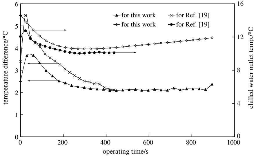
Fig. 11. Comparisons of the temperature difference between the chilled water outlet and the evaporating temperature and of the chilled water outlet temperatures.
