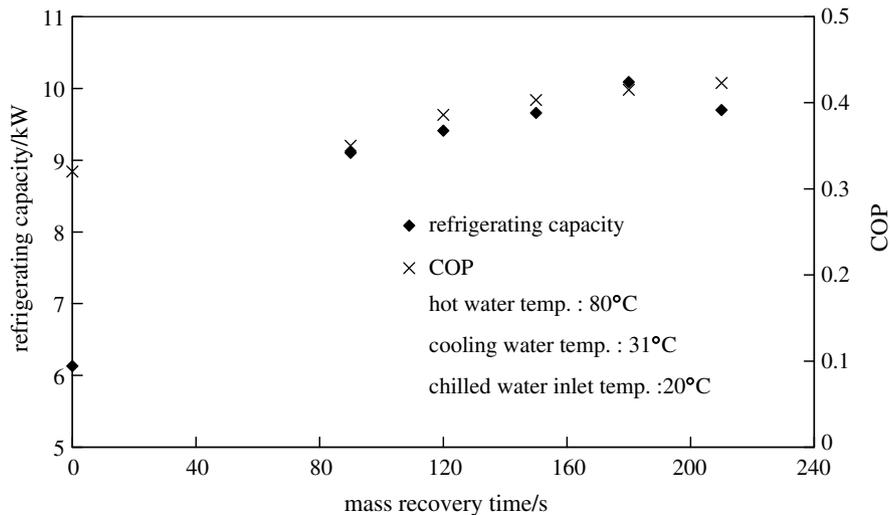
Fig. 7. Refrigerating capacity and COP variations with the mass recovery time.
