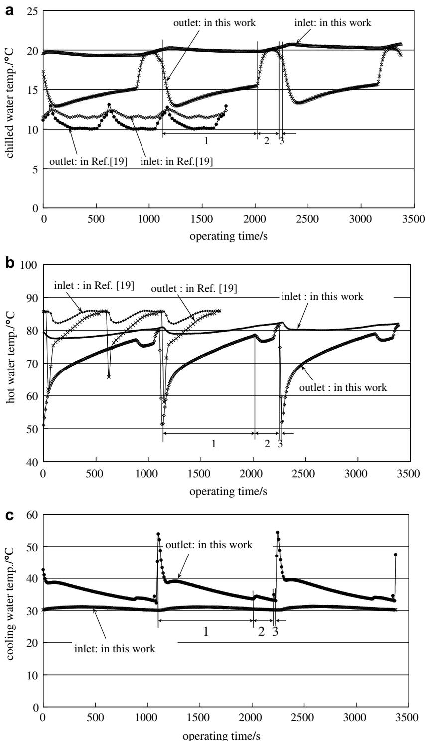
Fig. 6. Temperature variations of the hot water, cooling water and the chilled water (1, heating/cooling phase; 2, mass recovery phase; 3, heat recovery phase) (a) for chilled water, (b) for hot water and (c) for cooling water.
