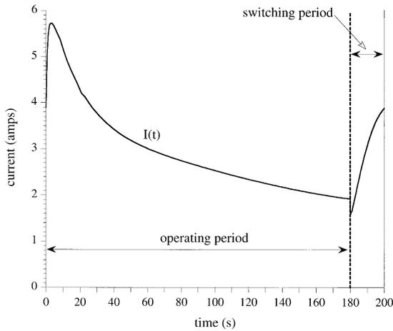
Fig. 4. The time evolution of input current during one chiller cycle at steady state. Cycle time = 200 s. Switching time = 20 s.
