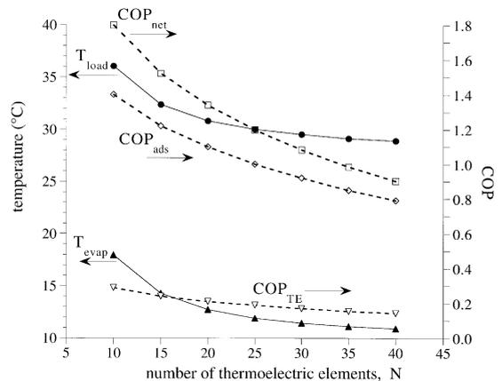
Fig. 6.  $T_{load}$ ,  $T_{evap}$ ,  $COP_{net}$ ,  $COP_{TE}$  and  $COP_{ads}$  as functions of the number of thermoelectric elements  $N$ .
