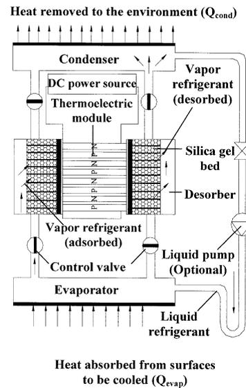
Fig. 3. Schematic showing the principal components and energy flows of the electro-adsorption chiller. The optional circulation pump is intended as a micro-electronic mechanical pump for highly miniaturized chillers, where condensate return action solely via a U-tube might be acutely sensitive to orientation changes.
