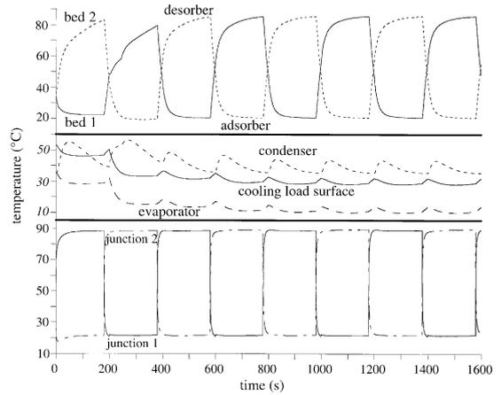
Fig. 5. Temperatures of the principal components as functions of time from initial start-up through cyclic steady-state. Cycle time = 200 s and switching time = 20 s. (a) Refrigerant in the two beds (alternating as adsorber and desorber). (b) Refrigerant in the condenser and evaporator, as well as the cooling load surface. (c) The two thermoelectric junctions (alternating hot and cold).
