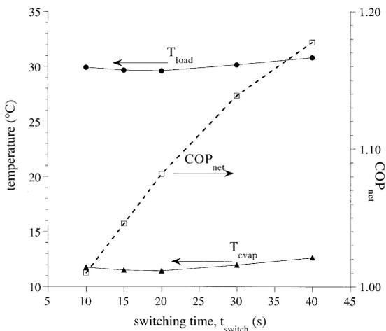
Fig. 8.  $T_{load}$ ,  $T_{evap}$  and  $COP_{net}$  as functions of switching time for cycle time  $\tau=200$  s.
