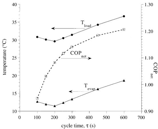
Fig. 7.  $COP_{net}$ ,  $T_{load}$  and  $T_{evap}$  as functions of cycle time  $\tau$ .
