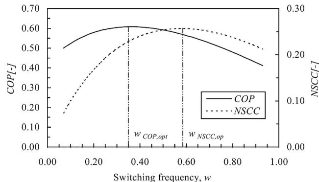
Fig. 2. COP and NSCC versus switching frequency,  $w$  for base run case.
