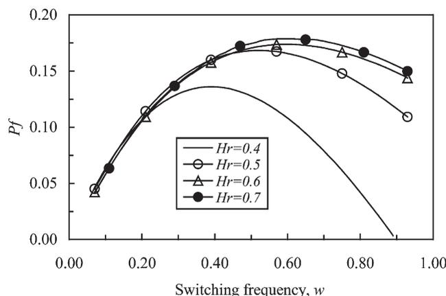
Fig. 7. Pf versus switching frequency,  $w$  for different Hr.
