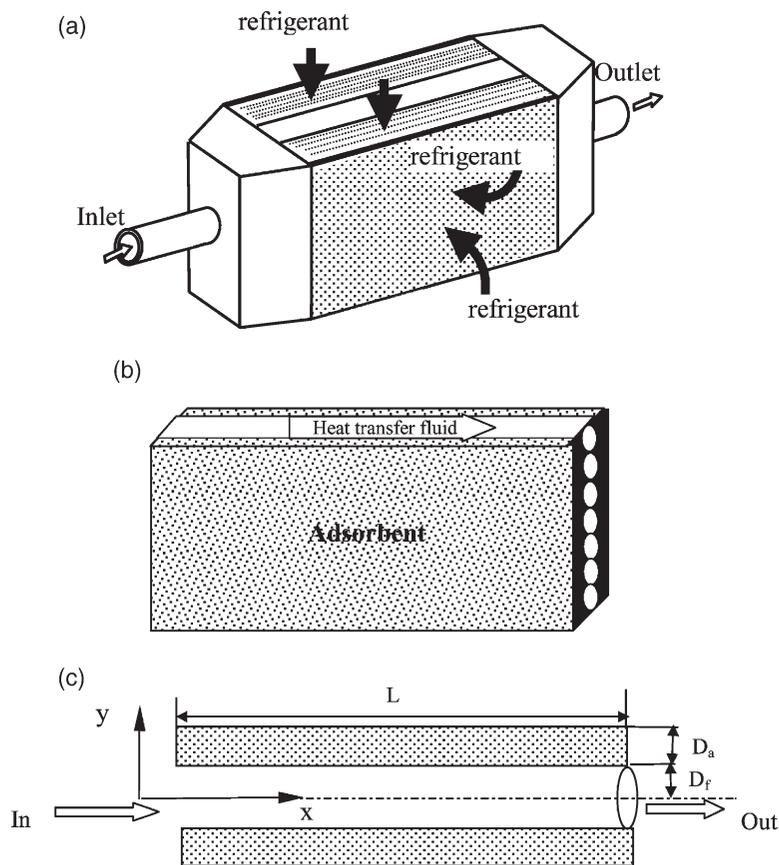
Fig. 1. (a) Schematic of an adsorbent bed heat exchanger; (b) schematic of side view of the adsorbent bed heat exchanger; (c) schematic of a flow channel.
